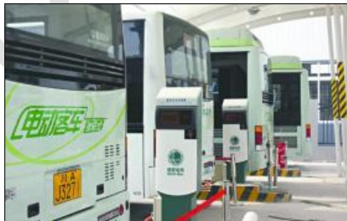
**Figure 14: Electric Bus Charging Stations**
